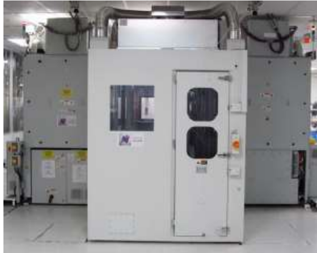
Figure 16: Tool for fast deposition of epitaxial layers of silicon based on atmospheric pressure chemical vapor deposition to produce thin epitaxial wafers for next generation solar cells
