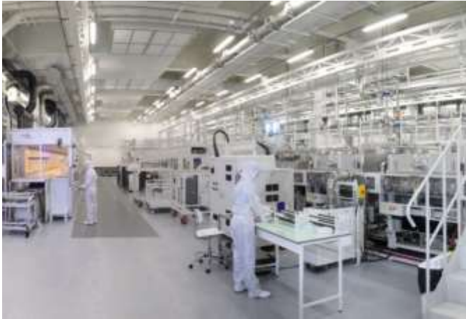
Figure 13: Left: typical view of technology development line with a capacity of realizing some thousands of solar cells per day. Right: A typical screen printer metallization tool for the solar cell pilot line
