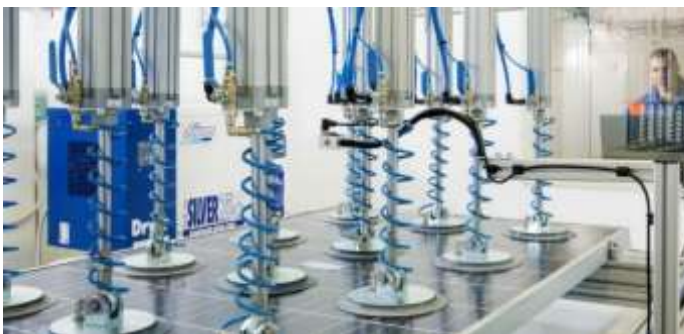
Figure 15: Left PV Modules Mechanical load test tool. Right climatic chamber for aging tests on PV modules. Both tools are very important for reliability tests in a characterization Lab
