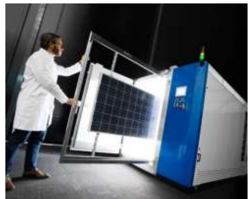
Figure 15: Left PV Modules Mechanical load test tool. Right climatic chamber for aging tests on PV modules. Both tools are very important for reliability tests in a characterization Lab
